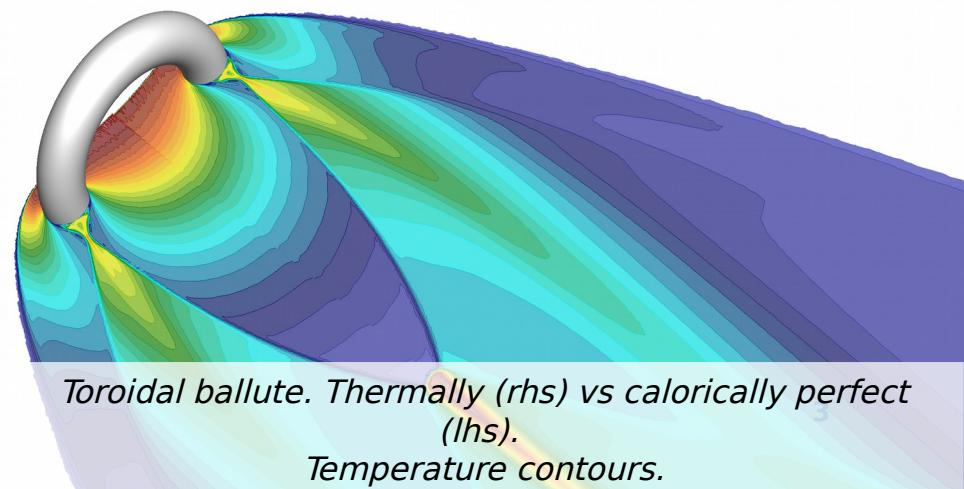
Toroidal ballute. Thermally (rhs) vs calorically perfect (lhs). Temperature contours.
