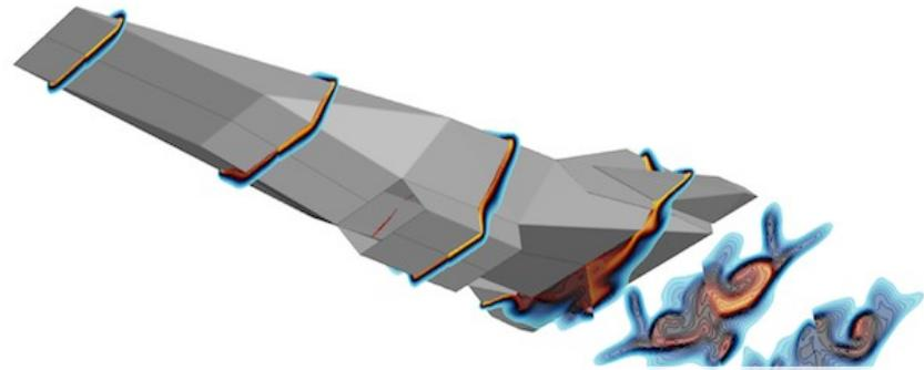
X43 vehicle. Thermally (rhs) vs calorically perfect (lhs). Temperature contours.
