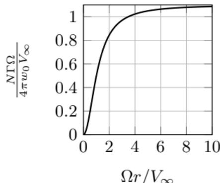
Non-dimensional circulation for the optimal propeller
