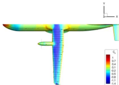
12 million grid elements (half configuration). Symmetrical flow for CPU saving implies counter-rotating propellers.
