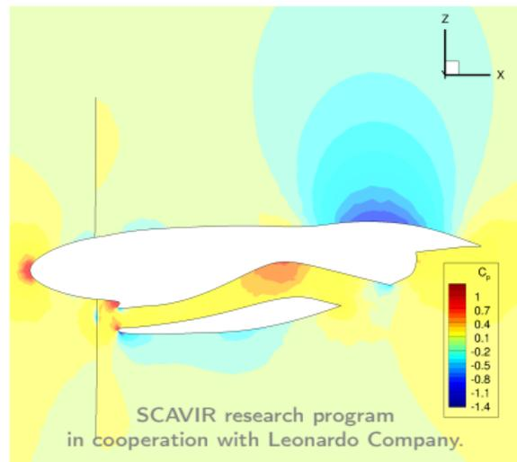
Pressure Coefficient Contour at nacelle symmetry plane
