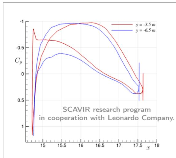
Pressure Coefficient distributions along 2 wing sections in the propeller streamtube.
