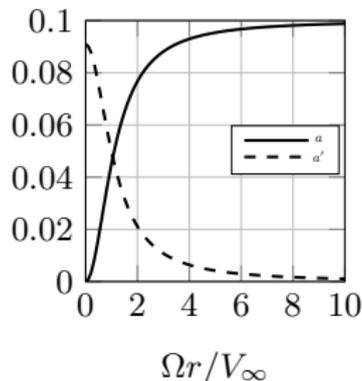
Axial and rotational interference factors for the optimal propeller
