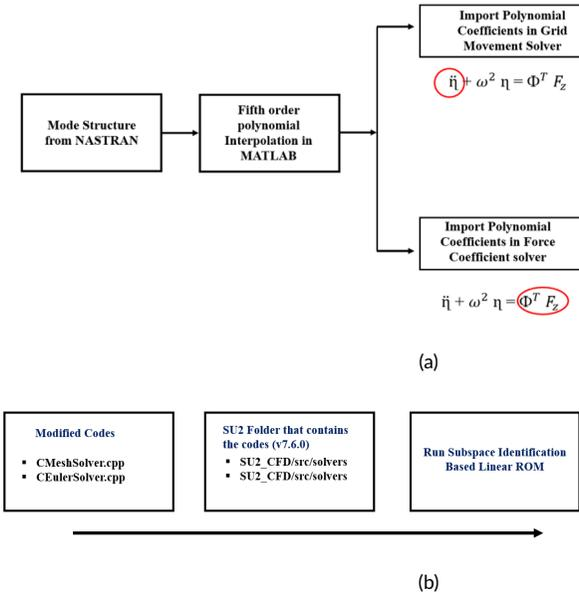
**FIGURE 1** (a) Implementation in SU2 (b) Modification of the SU2 solver (Mesh movement solver and the Force computation solver)
