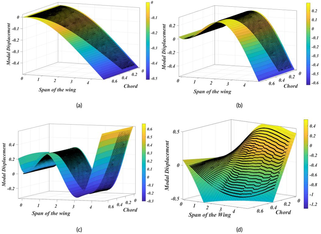
**FIGURE 2** Interpolation of the structural modes in the MATLAB platform (a) First Mode (b) Second Mode (c) Third Mode and (d) Fourth Mode.
