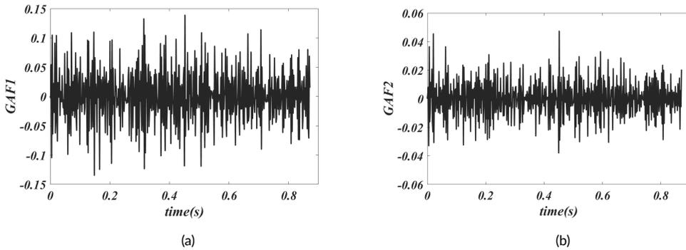
**FIGURE 4** Generalized aerodynamic force (a) GAF1 and (b) GAF2 under combined mode I and mode II interaction.
