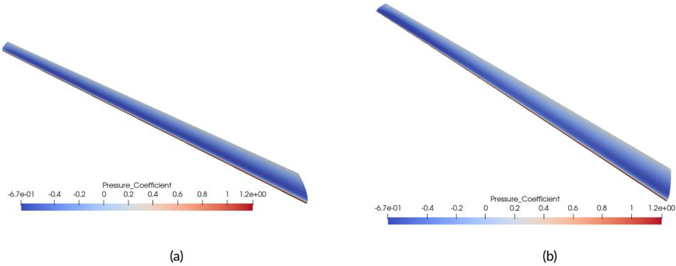
**FIGURE 3** The wing deflected at the maximum sinusoidal location under (a) first and (b) second mode excitation.
