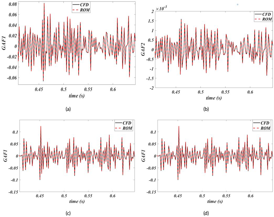
**FIGURE 6** (a) GAF1 and (b) GAF2 under mode I excitation (c) GAF1 and (d) GAF2 under mode II excitation randomly.
